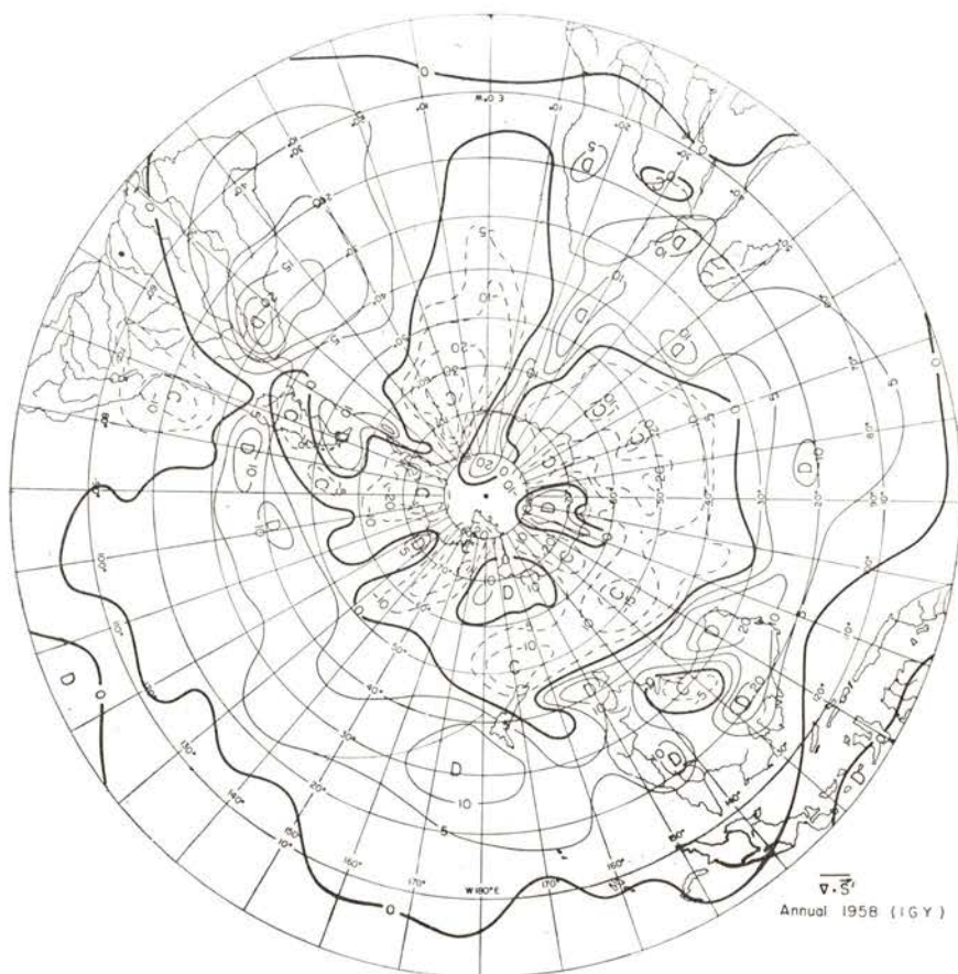
Fig. 1 — Mean annual distribution of the horizontal divergence of the vertically integrated transient eddy flux of enthalpy in 10^{-3} calories per square centimeter per minute.
