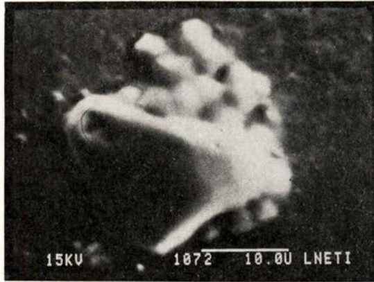
Fig. 6 — SEM micrograph showing an aggregate of iron particles.
