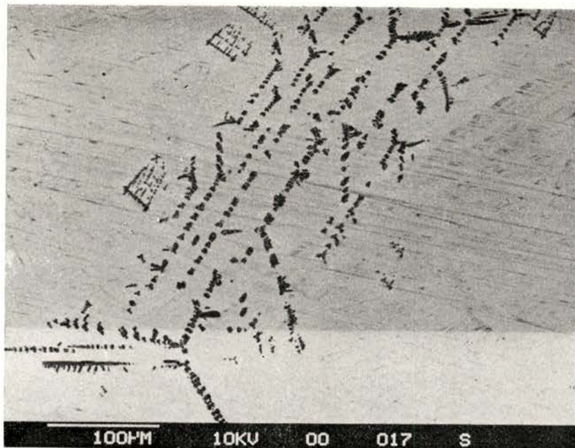
Fig. 3 — An «island» formed by crystals is seen, but the overall concentration is very small and X-rays do not «see» the crystals ( x = 0.4 ) ( \times 200 )
