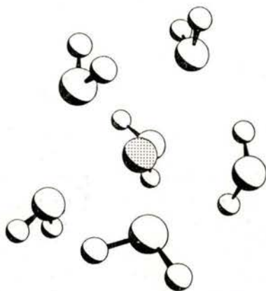
Fig. 2 — Snapshot of the \text{Li}^+ ion and its nearest environment from an MD simulation of a 0.43 M aqueous solution of \text{LiHCOO} at 300K [27].
